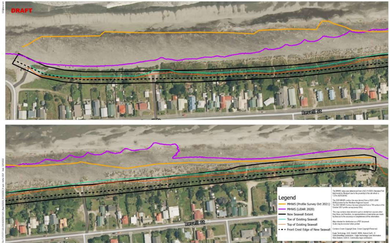
Figure 3-5 Proposed seawall extension footprint relative to MHWS
