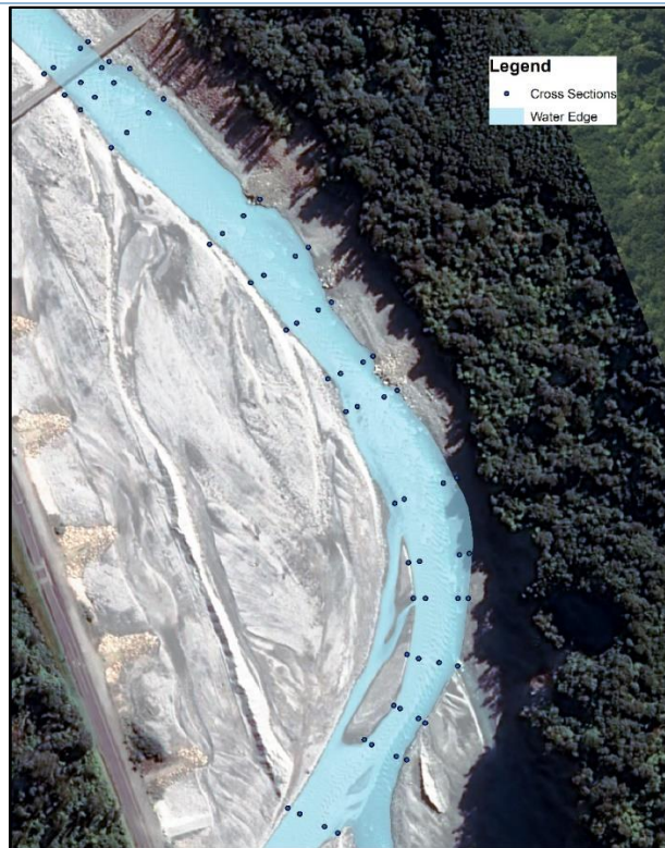
Figure 5-3 - Example of cross section locations in relation to main channel
