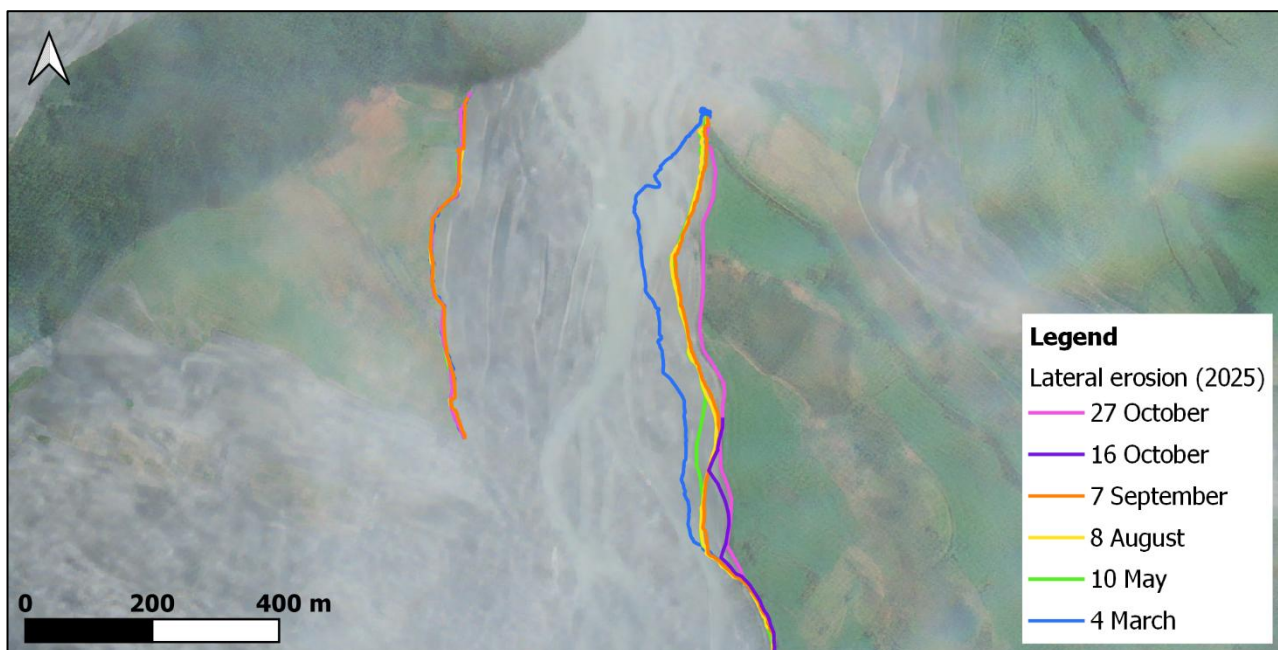
Figure 2-4: High resolution satellite imagery from 27 th October (after the LiDAR) shows further erosion.
