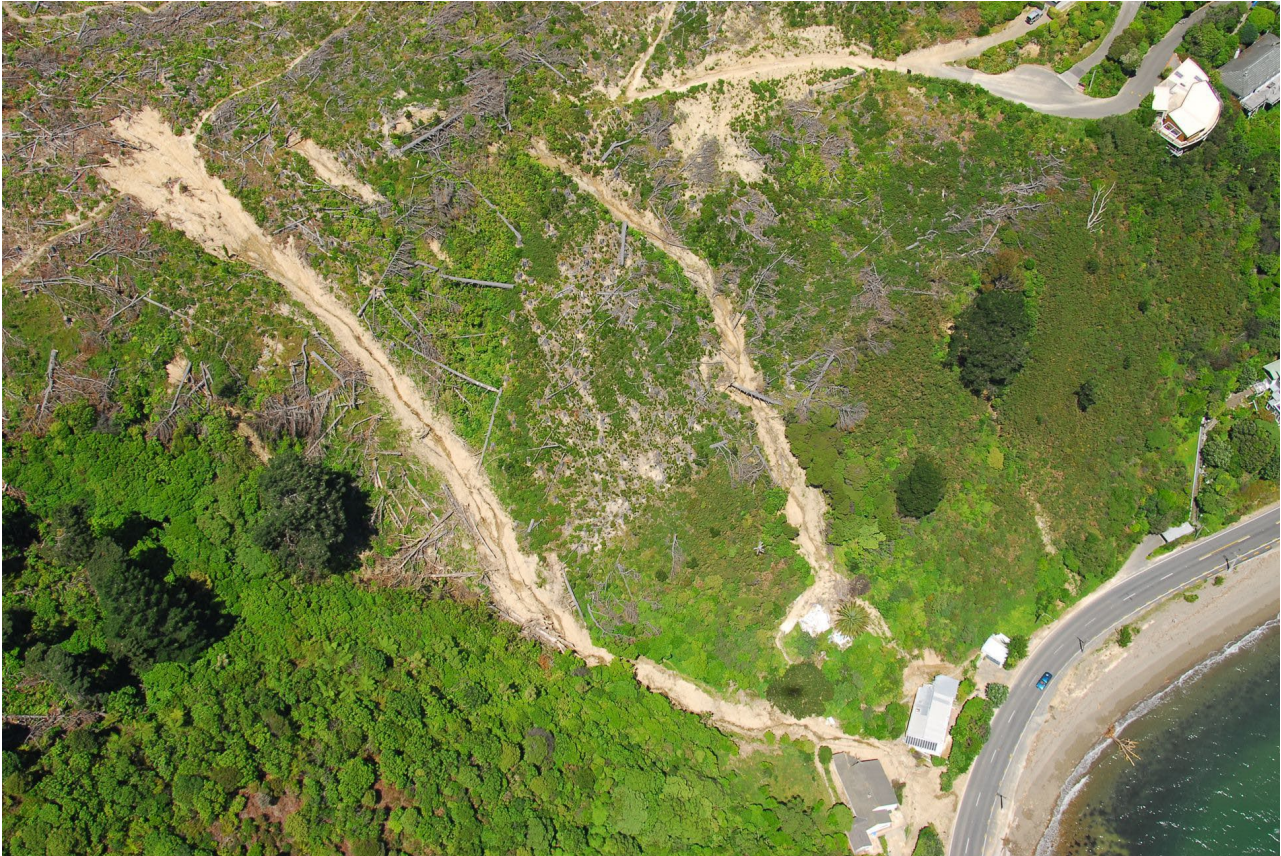
Figure 1.3 Debris flows generated by rain in Eastbourne, Wellington, in November 2006. The source areas of the debris flows are in the left of the photograph. The debris travelled down-slope several hundreds of metres, where it impacted the dwellings shown in the right of the photograph. Photograph by G Hancox, GNS Science.
