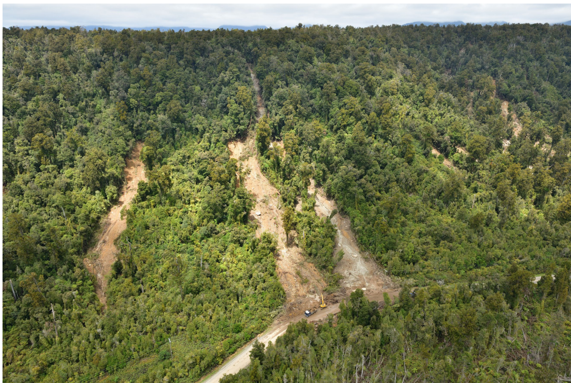
Figure 1.4 Debris avalanches on Whataroa Highway generated by the 2019 West Coast storm. Photograph by D Townsend, Earth Sciences New Zealand.
