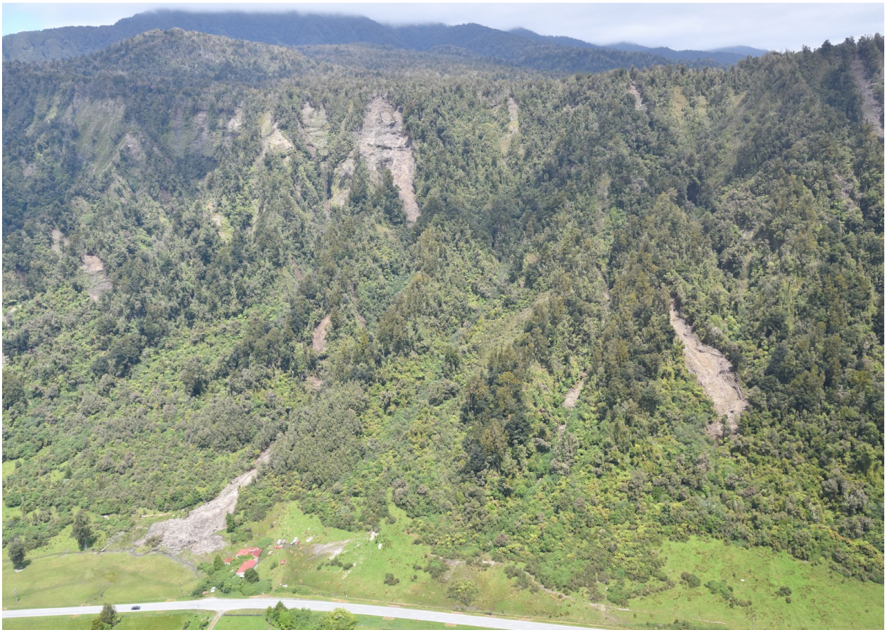
Figure 2.10 Landslides and debris flows generated by the December 2019 West Coast storm. The property in the foreground has a calculated present-day APLR of 5.3%. The calculated APLR for an RCP6 scenario is 5.7%. The risk from earthquake-induced flow-type movements is similar. There is no risk associated with avalanche-type movements from either earthquake- or rainfall-induced landslide events, as these do not travel as far as the property's location. We note that this assessment is based on a regional analysis and refer readers to Section 5.5 for further details on site-specific considerations. (Photo credit D Townsend, Earth Sciences New Zealand).
