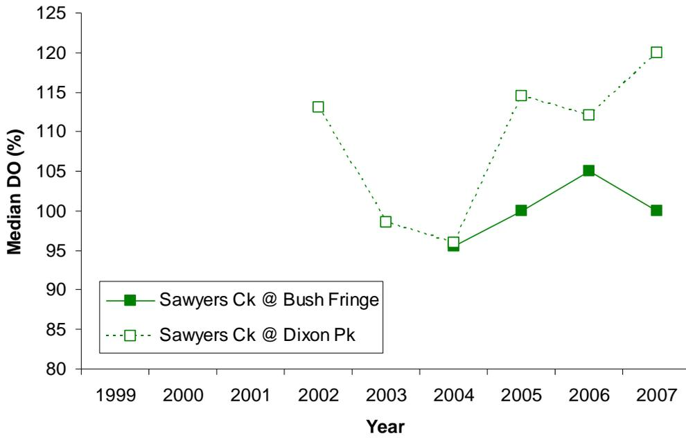
Figure 5.8.20 Sawyers Creek – Yearly median percentage dissolved oxygen saturation.
