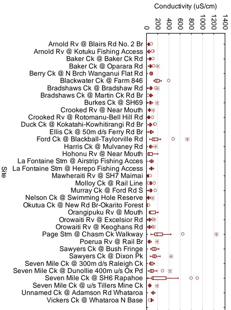
Figure 5.7.11 Box and whisker plot: Conductivity.
