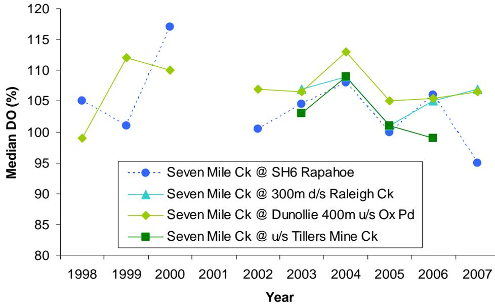
Figure 5.8.34 Seven Mile Creek – Yearly median percentage dissolved oxygen saturation.
