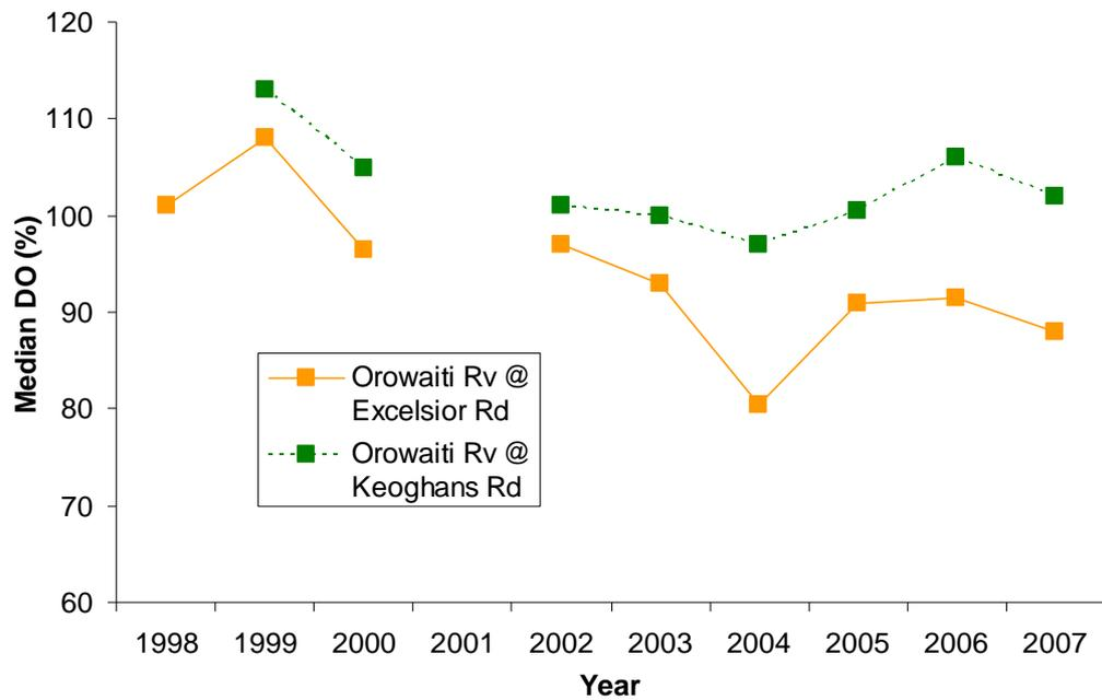
Figure 5.8.6 Orowaiti River – Yearly median percentage dissolved oxygen saturation.
