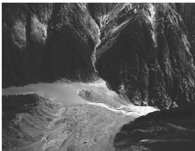
Fig. 2. Aerial view of Poerua landslide dam and lake on October 8, 1999. At this point, the lake is at its highest level (approximately 480 m), with an overflow channel established on the true left side of the dam and flowing into the Poerua River (Hancox et al. 2005).
