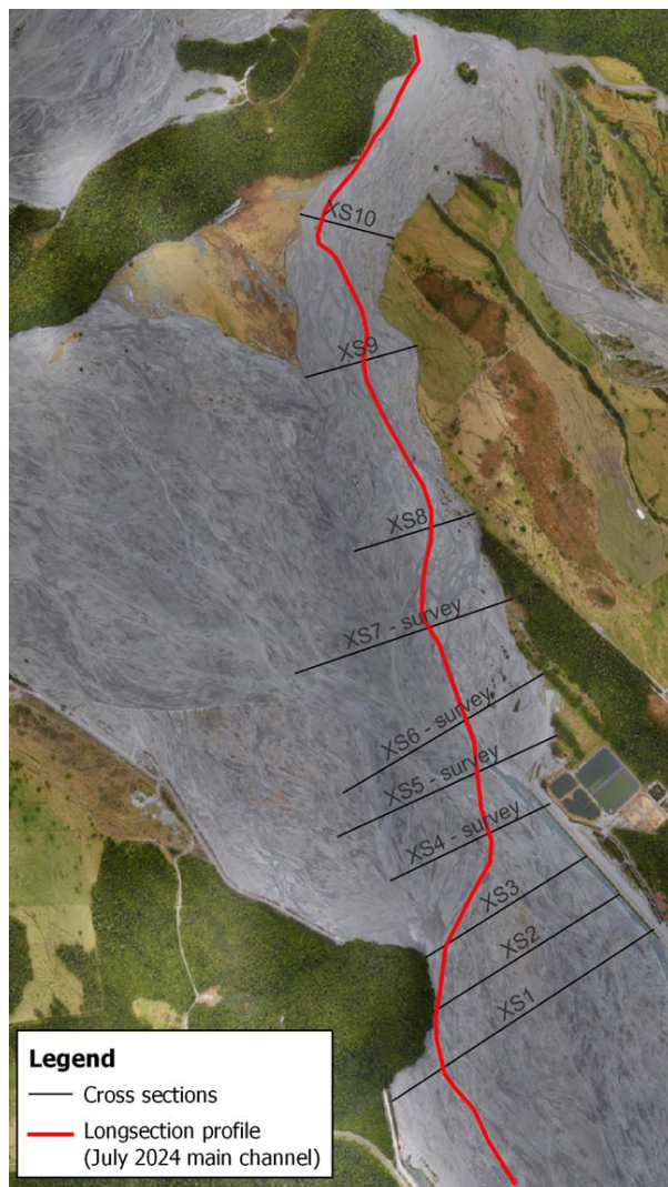
Figure 2-7 - Longsection profile down the July 2024 main channel, however, between 0 and 1300 m one of the deeper (dry) braids on the true left has been followed.
