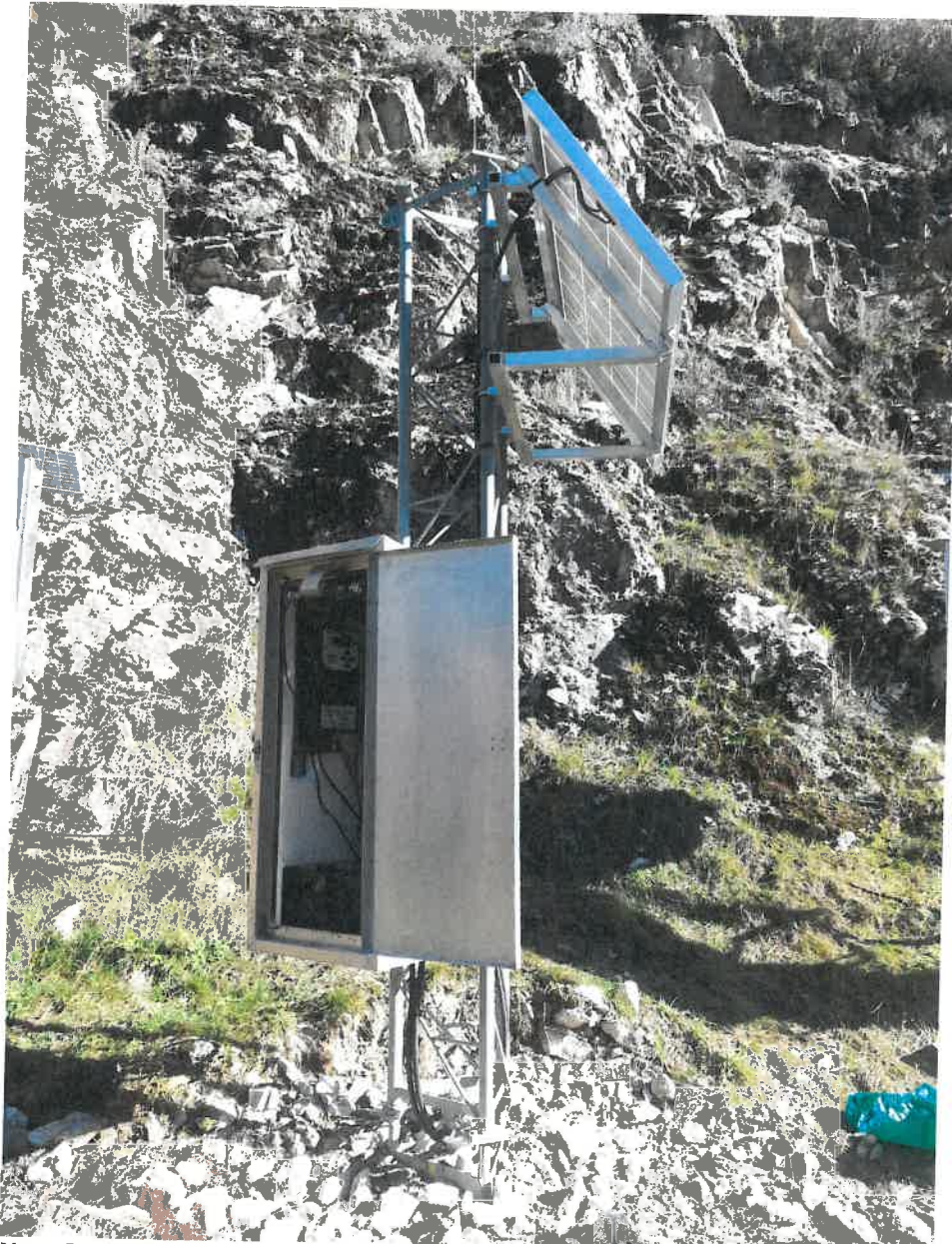
New Grey River at Waipuna recorder box and tower (with solar panel and aerial)
