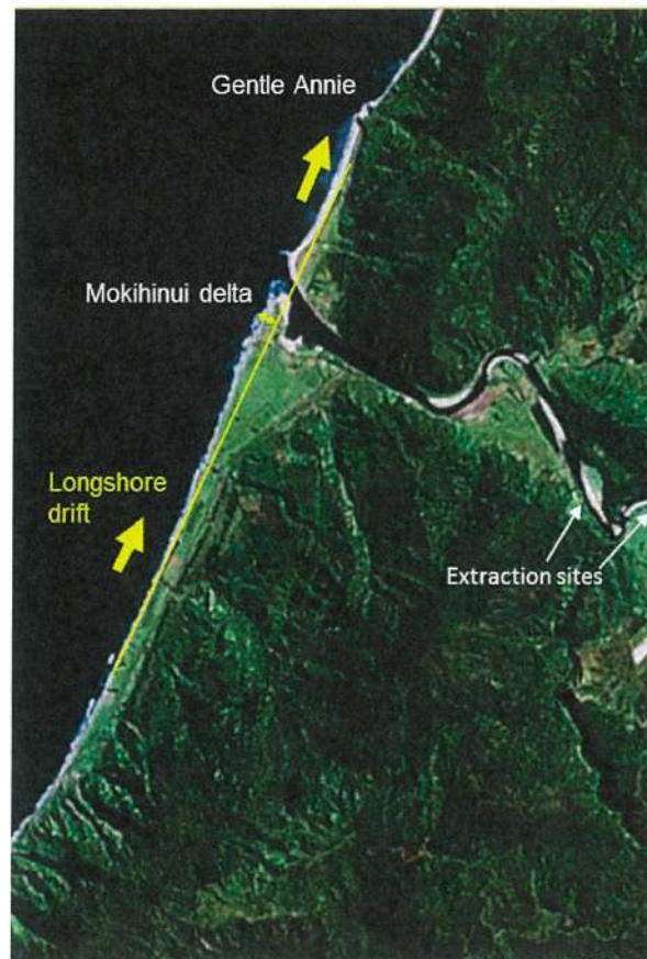
Figure 2-1: Mokihinui River mouth. The wave-dominated delta at the Mokihinui River mouth traps littoral drift sand moving alongshore from the south, stocking the beach south of the river mouth. Yellow line indicates extent of shoreline extension by river delta. Reducing the river’s sand and gravel load will ‘flatten’ the delta and cause the beach to the south to be trimmed back (potentially to yellow line).
