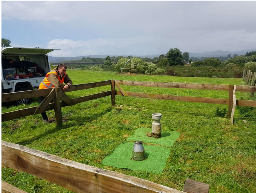
Figure 2: Hydrology Technician, Reuben, conducting a final inspection of monitoring site Mawheraiti River @ Atarau Bridge where artificial grass has been installed around gauges to reduce the impact of grass growth on measurements.
