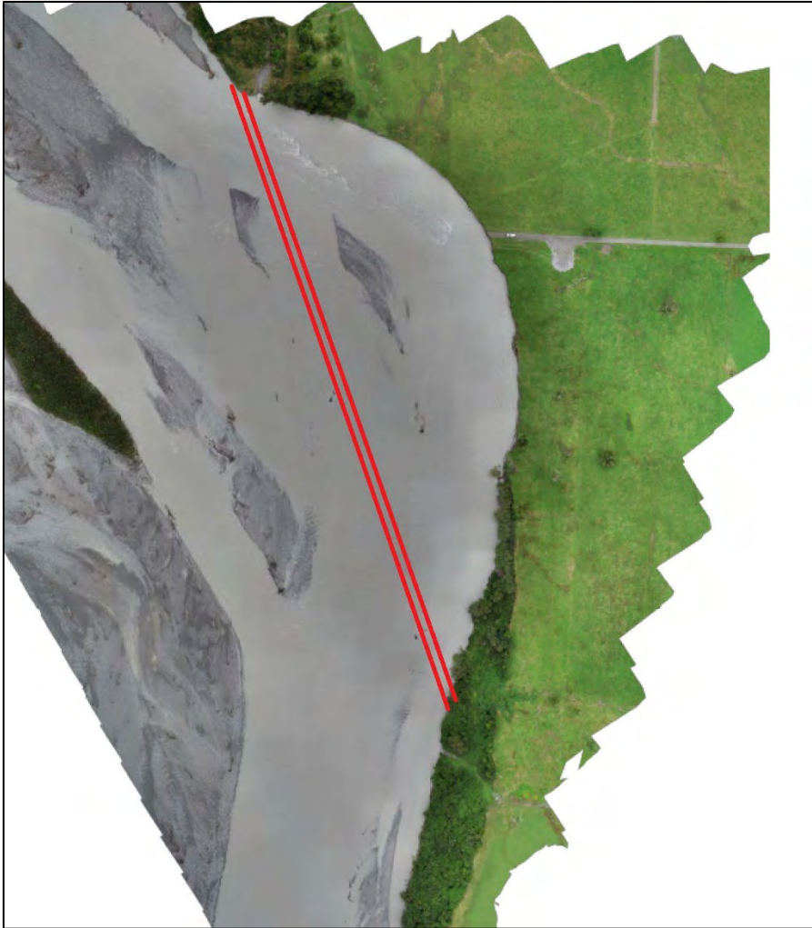
Drone view of Damage and Alignment of proposed low height stop bank
