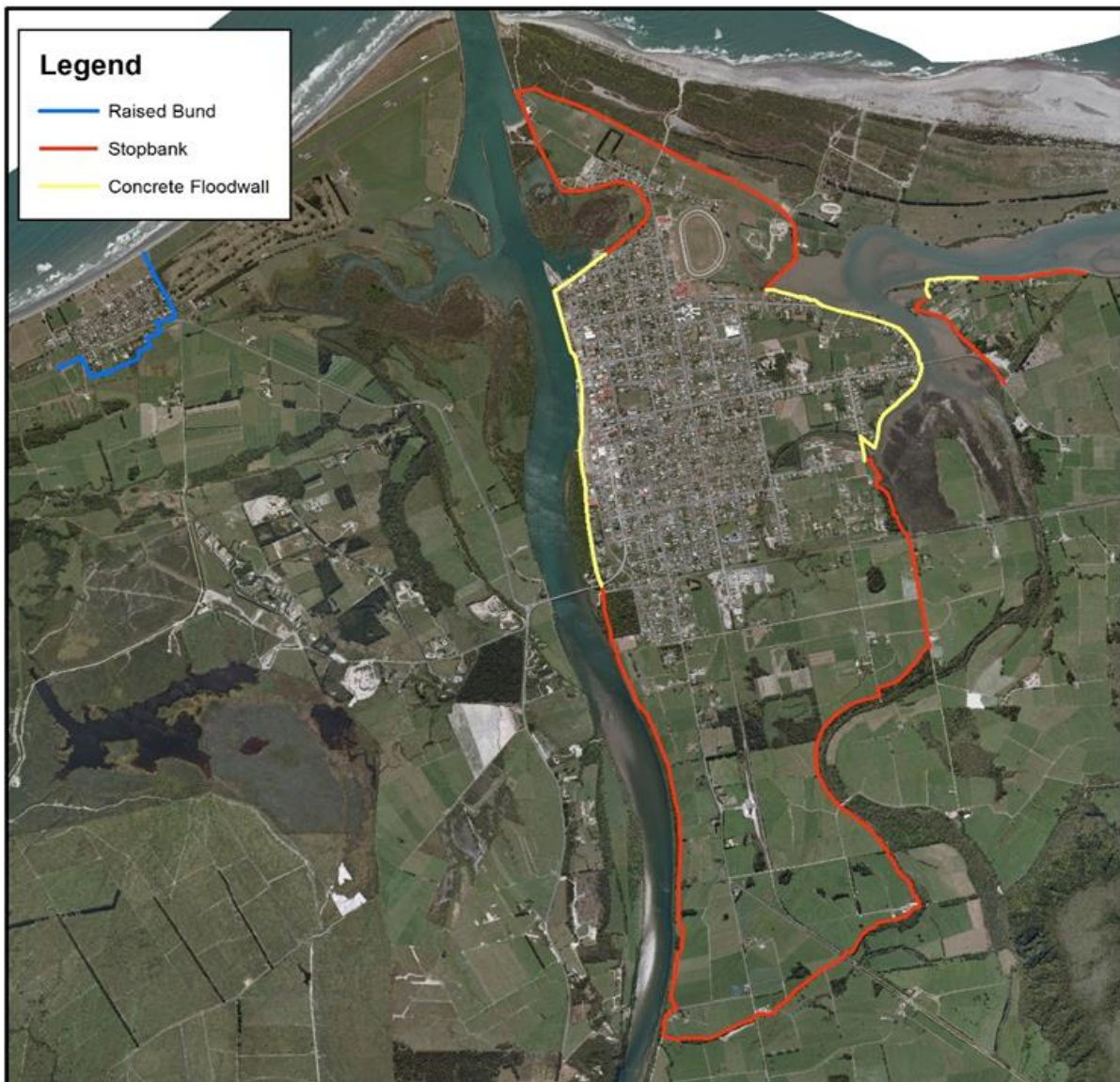
Figure nine: proposed flood protection structures for Westport. Source: West Coast Regional Council.
