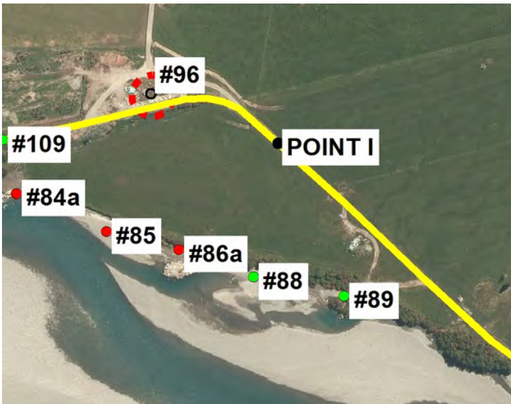
Site 1 - Damage to Asset #88 requiring 240 tonnes of rock to remedy
