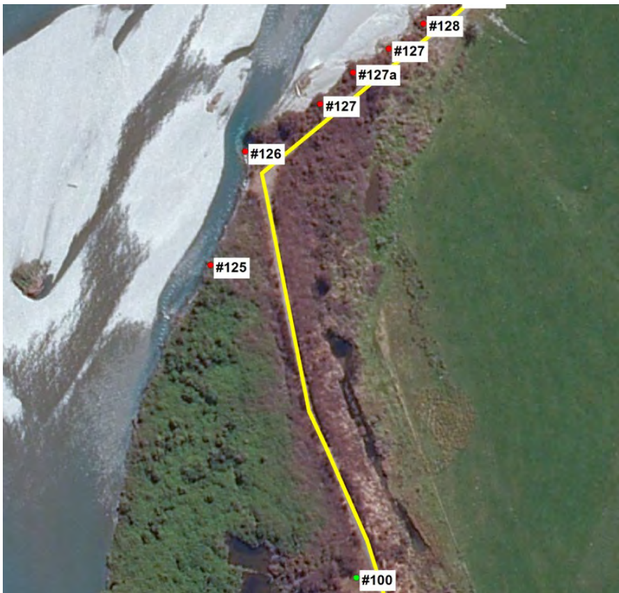
Site 2 – Damaged to Asset #126 to #100 requiring 440 tonnes of rock to remedy
