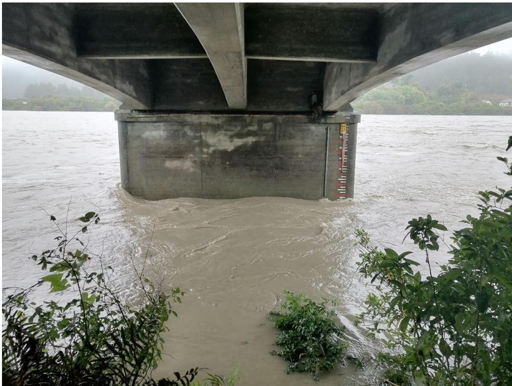
Staff gauge at the Hokitika Rv at Kaniere Bridge site at 09:45am 21 st April (peak was at 09:40am)
