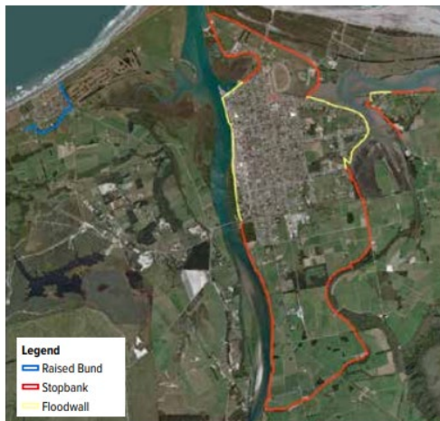
Figure 9: Option 2 - Extensive stopbanks and flood wall scheme
