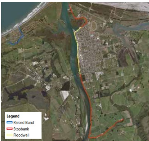
Figure 8: Option 1 - Partial stopbanks and flood wall scheme
