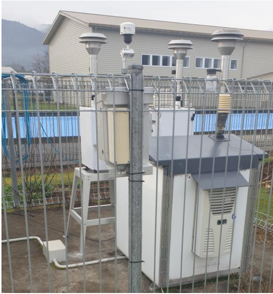
Figure 3: Photograph of an ES642 unit collocated alongside the WCRC instruments at Reefton.
