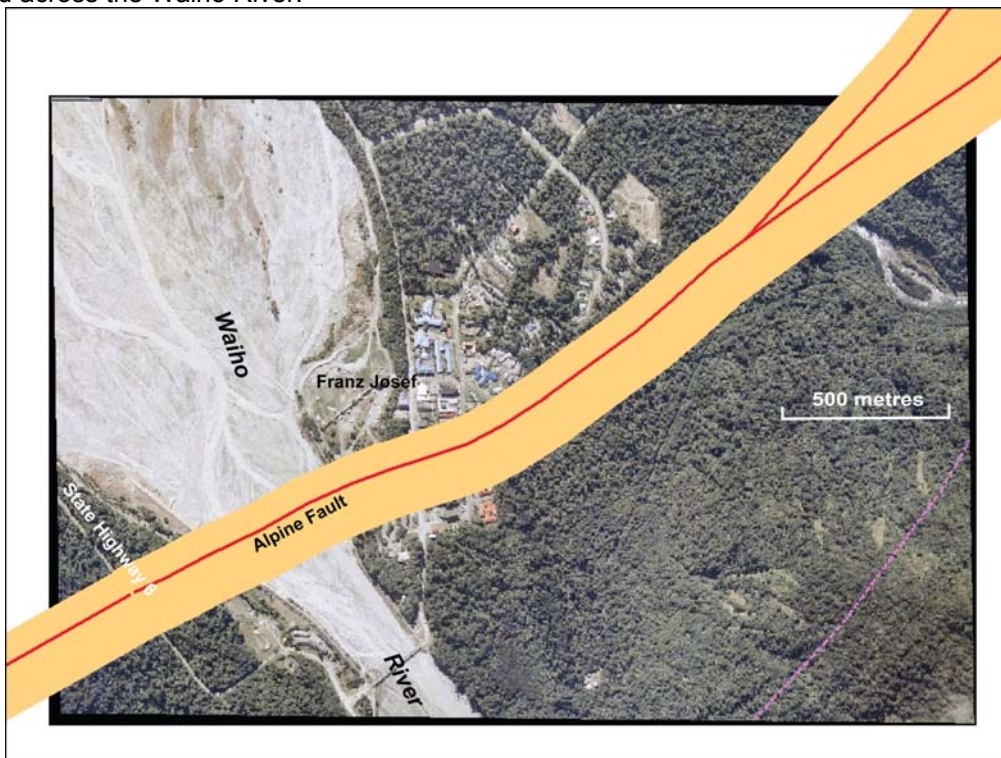
Figure 20 The Fault Avoidance Zone (FAZ) for the Alpine Fault in the Franz Josef area (scale extracted from GIS at 1:9000). Both the new mapped fault trace and the dashed WCRC line occur within the FAZ. In terms of future mapping and consenting, a zone of width of 190m is currently placed through the town until better mapping data becomes available.
