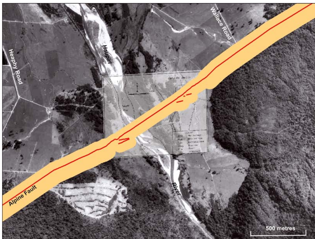
Figure 14 The Fault Avoidance Zone (FAZ) applied to the trace of the Alpine Fault in the Haupiri River area (scale c. 1:10,000). The extent of the orange strip represents the FAZ results that are presented to WCRC in the GIS. In this example, secondary fault traces mapped by Yetton (2000) have been included and buffered separately to the main trace of the fault. Note how the total FAZ broadens about secondary traces.
