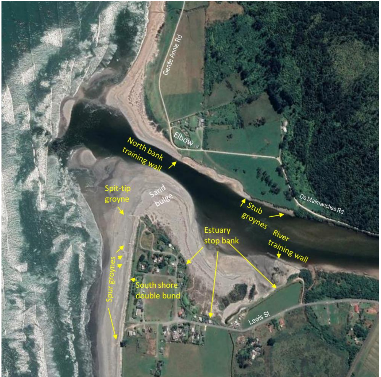
Figure 2-1: Photo-map locating structures at Mokihinui River mouth. Image from Google Earth (photographed 2018).
