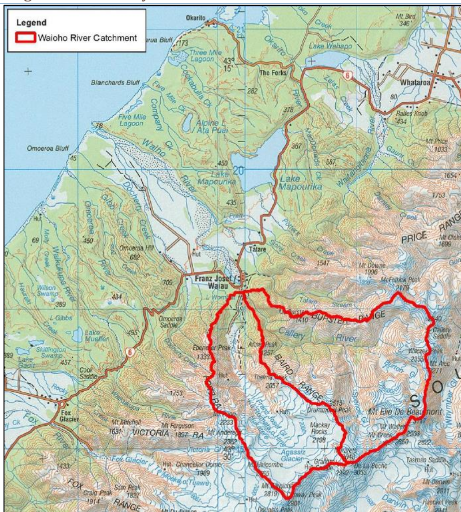
Figure 1-1 – Location map of the Waiho River highlighting the hydrological catchments for the Waiho River and the Callery River upstream of SH6 bridge
