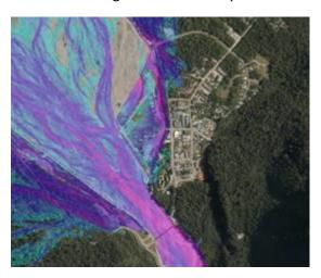
Figure 2-15: Flood model for 4m bed aggradation – 20-year, 1900 cumec flood
