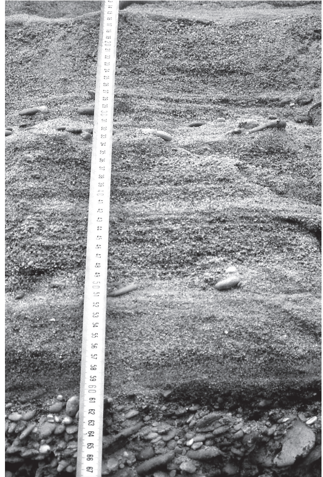
Fig. 6 Contact between Facies 5 gravels showing strong pebble imbrication and overlying sands of Facies 6 containing discontinuous pebble layers. View to east, scale in centimetres.
