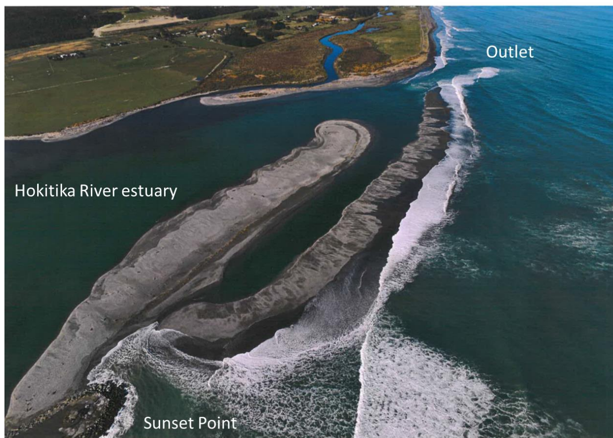
Figure 2-1: Bars partially blocking Hokitika River mouth, September 2015. View is to southwest. Note obliquely-approaching waves. Photograph supplied by WCRC.
