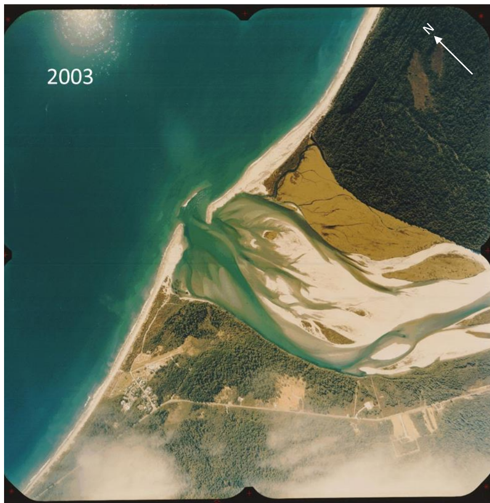
Figure 3-11: Neils Beach and Arawhata River mouth in 2003 and 2013. Note on 2013 image: flattened delta 'bulge', northward-displaced mouth, 'drumstick' growth on east side of river mouth, and right bank of river trimmed back.
