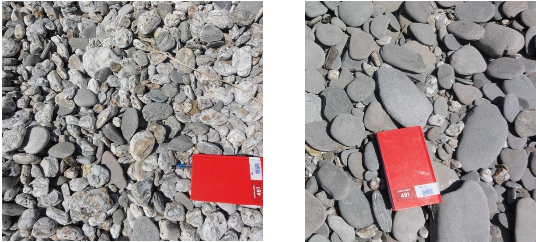
Figure 3-8: River and locally-sourced beach gravel on Neils Beach. Left shows mainly finer, rounded schist pebbles sourced from the Arawhata River. Right shows platy meta-sandstone pebbles and cobbles sourced from hillside gullies immediately west of Neils Beach.
