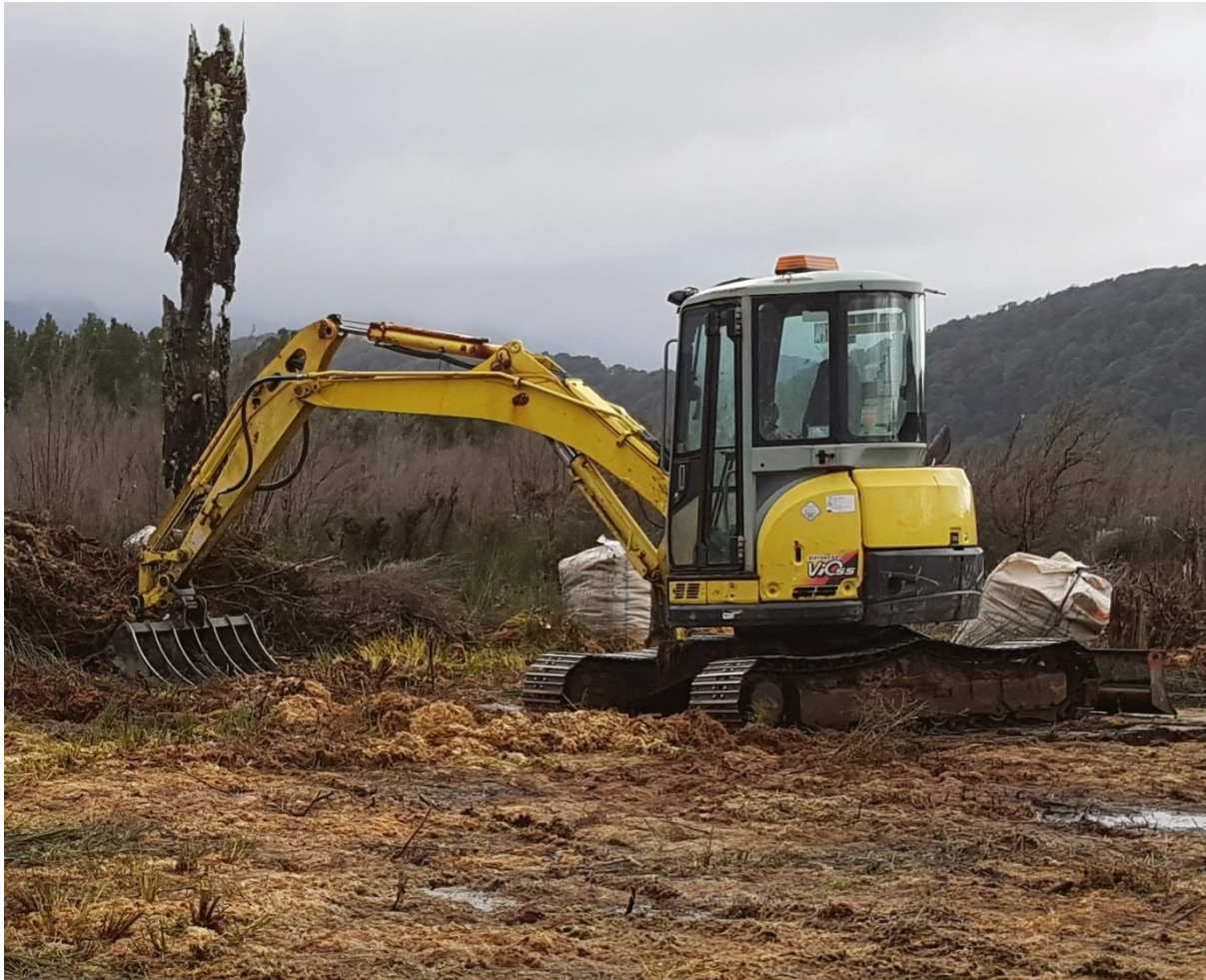
Figure 2. Heavy machinery supported by a wooden platform has less ground pressure than a person. The stump is a relic of historic forestry.
