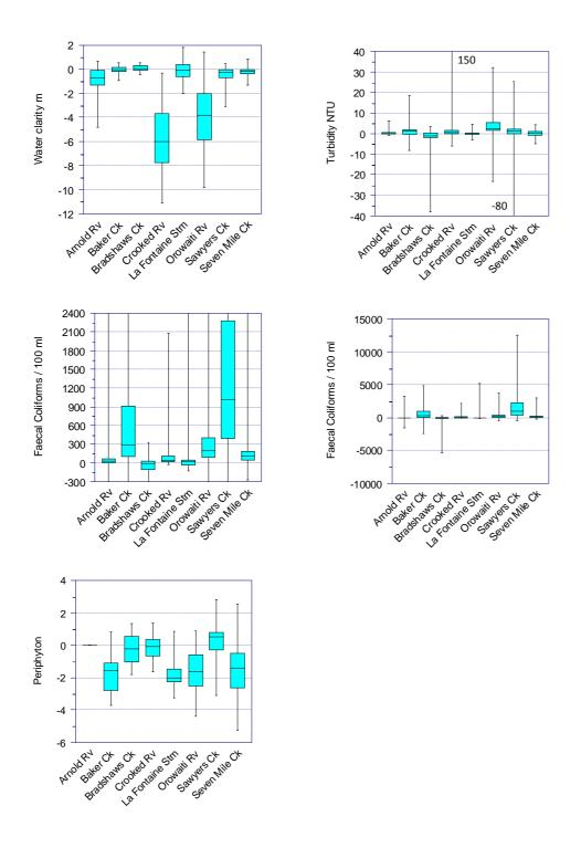
Figure 5.7.1b Differences between paired sites (upstream minus downstream values). Clarity, turbidity, faecal coliforms, and periphyton.
