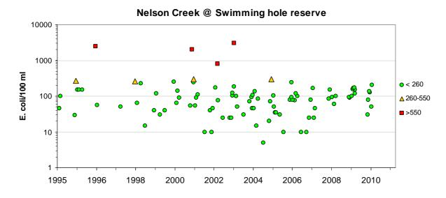
Figure 5.8.13 Single sample E. coli levels for Nelson Creek @ Swimming hole reserve.
