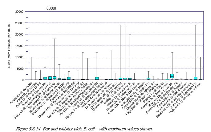
Figure 5.6.14 Box and whisker plot: E. coli – with maximum values shown.
