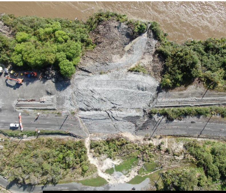
Omoto landslide State Highway 7 – aerial. More than two metres drop overnight in heavy rain – 19 October 2019
