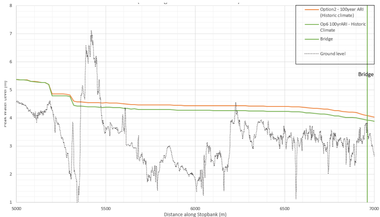
Figure 2-11 – Difference in stopbank crest levels upstream from the Orowaiti Bridge between Option 2 and Option 6 (100-year ARI – Historic Climate)
